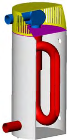
Figure 17. Condensing storage heater.
