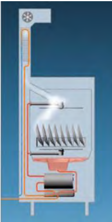
Figure 36. Diagram of integrated exhaust air and drainwater heat recovery in a door-type dishwasher. Photo Credit: Winterhalter
